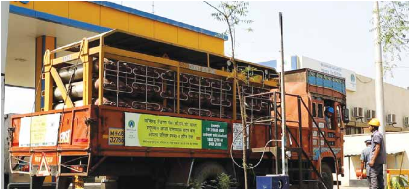
Filling of CNG Cascades.
